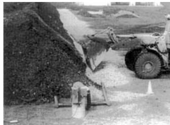
**The Com-Til Facility in Columbus, Ohio, composts biosolids. Wood chips, recycled compost and sawdust are added as bulking agents. The facility handles 50,000 wet tons of biosolids each year-25 dry tons per day. One eighth of the volume produced is sold as bagged compost and the remainder as bulk compost. The facility features an open concrete pad. Compost is piled 10- to 12-foot high on perforated plastic tile to achieve updraft aeration.**
